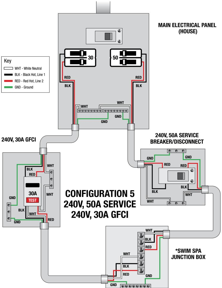
\*Refer to wiring diagram inside swim spa junction box for proper power connection to terminals. The swim spa junction box is located inside swim spa behind the factory installed GFCI. Remove skirt access panel "B" to gain access to swim spa junction box (see Glossary of Swim Spa Terminology).
