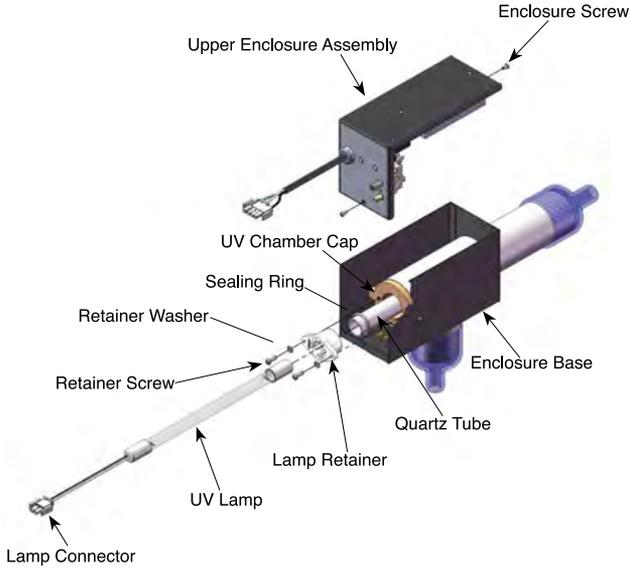
**Figure 2: Spa Solar Eclipse Exploded View**
